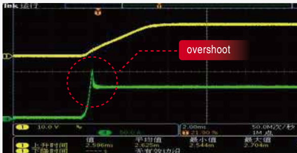
Diode load Conventional power test
