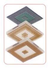
Andon Electronics announced the launch of their BGA Rollerball Sockets and Adapters. These Sockets and adaptors provide an ideal method for mounting ball grid array devices onto a PCB. The device is soldered to the adapter, greatly simplifying solder verification and testing. The device/adapter assembly then plugs into the BGA socket which is permanently soldered to the PCB.
